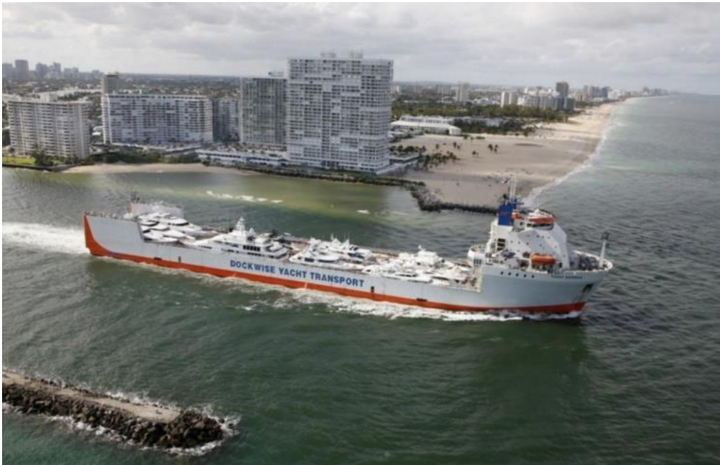
Figure 40 – Semi-Submersible Ship Fully Loaded 1
