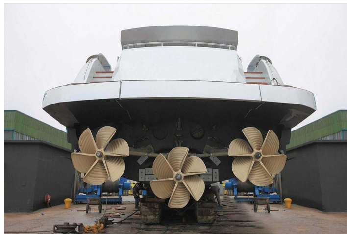
Figure 5 – A 108-foot Pershing Yacht With a Triple Surface Drives Setup
