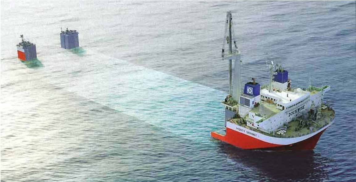
Figure 13 - Typical Float-on / Float-off Ship Ready to be Loaded
